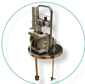
B24 and B24MIX are a pneumatic pumps with low air consumption. The valves are in stainless steel, the part of the diaphragms in contact with the fluid is in PTFE or polyamide and, thanks to the design and the accurate choice of components and materials, they are easy to service, providing a long working life.
